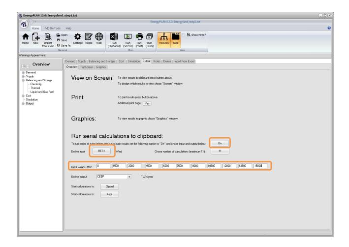
You can check how much electricity is produced from these various amounts of wind power, by going to the Input-RenewableEnergy tabsheet. For example, 15000 MW of wind produces 31.1 TWh of electricity, which is just over 100% (103.7%) of the electricity demand.
