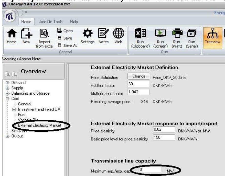
Set Transmission line capacity to zero
